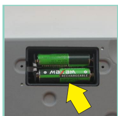
Container with accumulators
